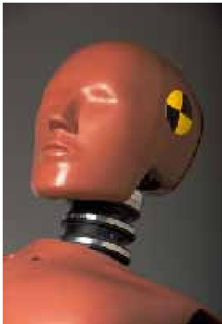
Fig. 4. Hybrid III dummy [21].
