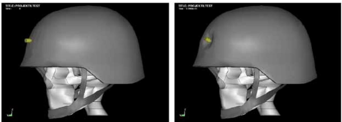
Fig. 2. A model of human head with a ballistic helmet before and during bullet impact [19]
